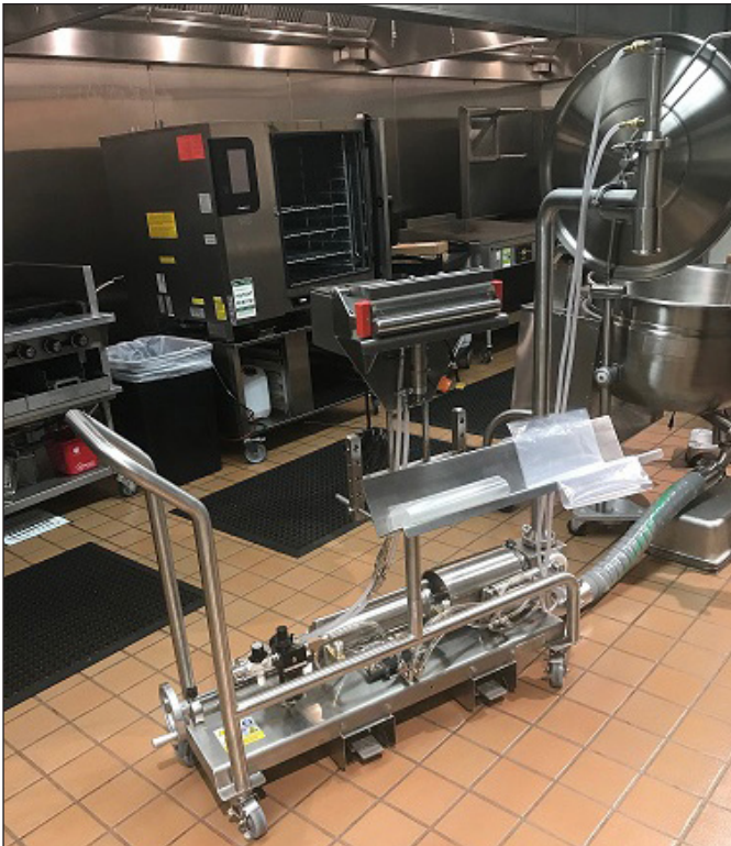
TEMPF-ECONO-YT (SHOWN ATTACHED TO EXISTING KETTLE)
