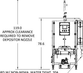
7' CORD W/ NON-NEMA, WATER TIGHT, 20A, 120/208V, 3 PHASE, 4 POLE, 4 WIRE PLUG – (CONNECTING FEMALE RECEPTACLE INCLUDED)
