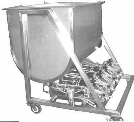
Pumps mounted to hopper rack
